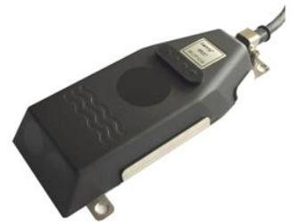
Ultraflow 6537 Velocity and Level Transducer is a unique combination of water velocity, depth, pressure, conductivity and temperature instruments integrated with a solid state logger. It is a new generation of intelligent flow measurement systems.
